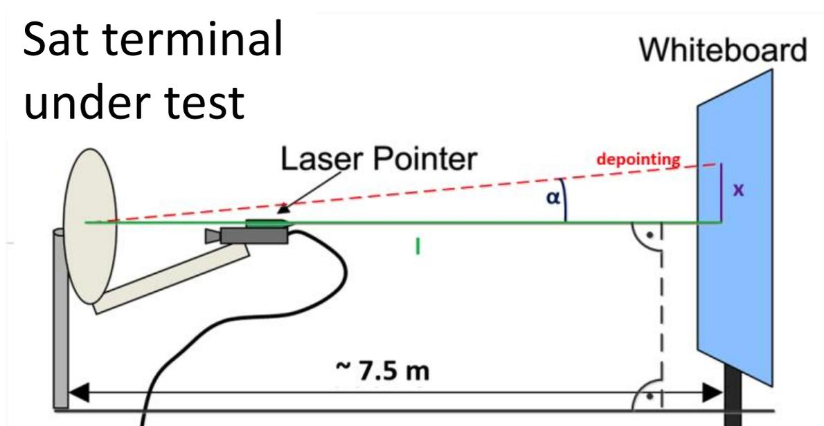
Figure 11-2: de-pointing tests using a laser pointer
